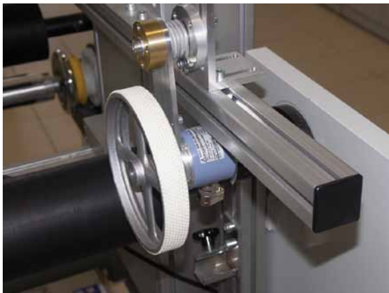
Image 6 - The encoder will be delivered completely with measuring wheel and spring lever 1
